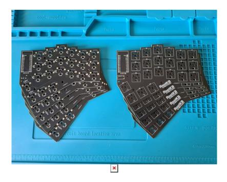
It was time to build the keyboard. I soldered all the 44 diodes, 44 switch sockets and 44 LEDs. For socketing the microcontrollers I used resistor legs as pins in order to fit the case as mentioned above.
