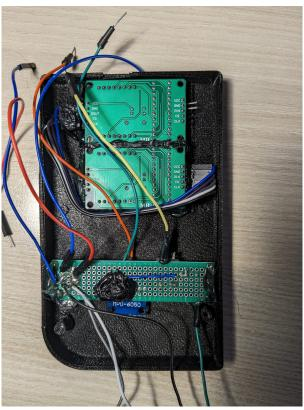
The project is coming along pretty well. Most of the pieces fit well together. I group bundles of wires that are close together and bundle them up. Essentially making my own custom connectors (Primitive in appearance but functional. This makes it easier to remove the Arduino if needed).
