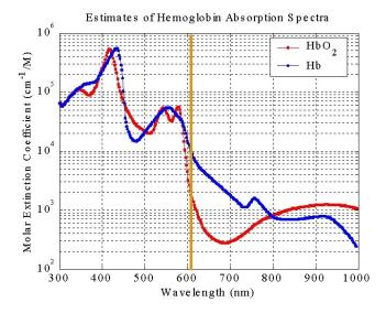
The processor calculates the ratio between the measurements of red and infrared light, and then utilizes a lookup table based on the Beer-Lambert law to convert it into SpO2 (oxygen saturation).
