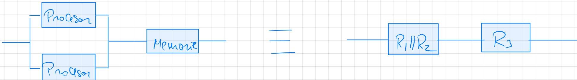
$$R_1, R_2, R_3 \rightarrow R_{TOTAL} = (R_1 \parallel R_2) \cdot R_3 = (1 - (1 - R_1)(1 - R_2)) \cdot R_3$$
