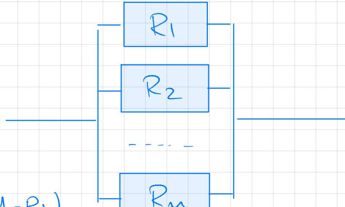
$$R_{\text{parallel}} = 1 - Q_{\text{parallel}} = 1 - \prod_{i=1}^n Q_i = 1 - \prod_{i=1}^n (1 - R_i)$$
