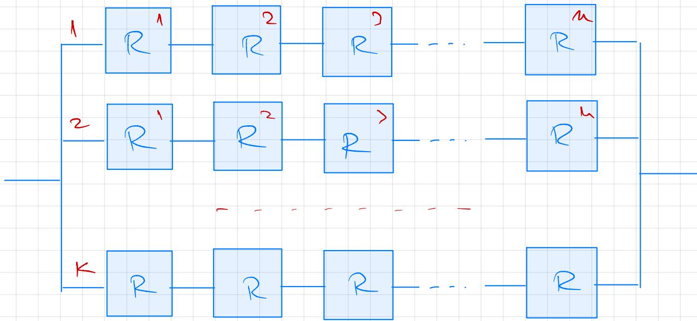
$$R_{SP}(t) = \underbrace{R^u || R^n || \dots || R^n}_{k ori} = 1 - (1 - R^u(t))^k$$
