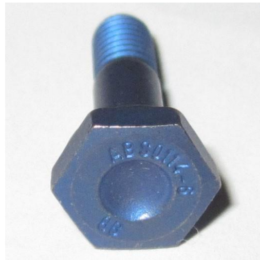
Airbus A-380 bolt with part tracking information. (Size: 2 cm x 1 cm)
