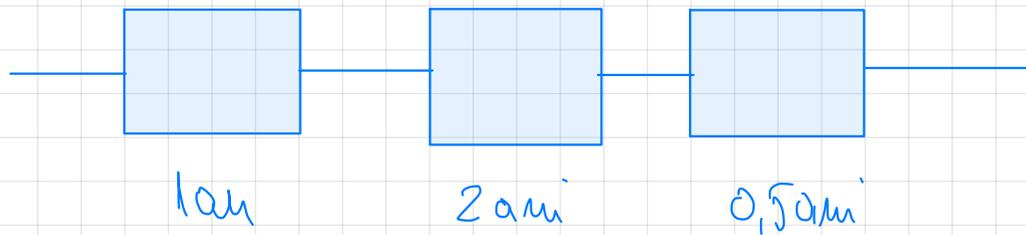
$$MTBF_S = \frac{1}{\frac{1}{1} + \frac{1}{2} + \frac{1}{0,5}} = \frac{1}{3 + \frac{1}{2}} = \frac{2}{7} \text{ an} = 0,28 \text{ an}$$
