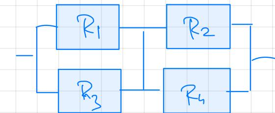
$$R_{C_2}(S | \bar{R}_5) = (R_1 R_2) || R_3 R_4 = R_1 R_2 + R_3 R_4 - R_1 R_2 R_3 R_4$$
