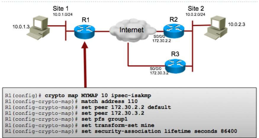
Multiple peers can be specified for redundancy.
