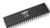
MOS 6502 (1975) 1 – 4 MHz Apple I & II, BBC Micro, Atari VCS, Nintendo NES, Commodore 64, and many early arcade machines
