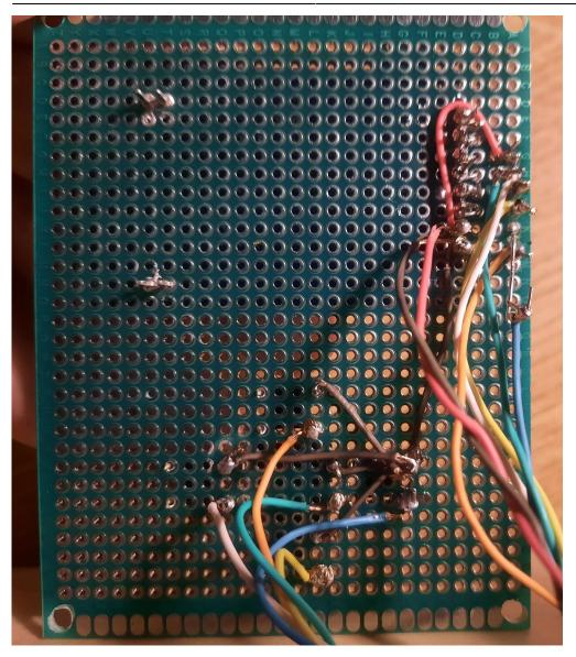
The front panel board is wired according to the schematic. The sound and power board has both the DFPlayer and the amplifier wired to it, in addition to the DC power jack 9V battery input and the 5V power rails where all the devices draw power from.
