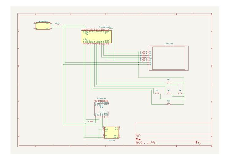
The schematic is representative of the final product, however the battery and the speakers have not been represented, and the connections to the button pins may not be identical. The pinout of the Arduino is visually that of a Nano, however the final product uses an Arduino Uno.
