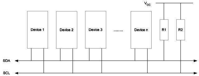
The TWI bus is a multi-master bus where one or more devices are capable of taking control of the bus, can be connected. Only Master devices can drive both the SCL and SDA lines, while a Slave device is only allowed to issue data on the SDA line.
