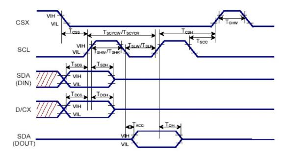
Table 17.3.2.2: 4 pin Serial Interface Characteristics
