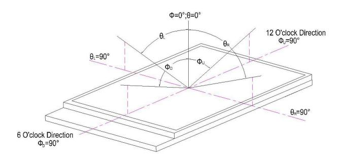
FIG.4 The definition of Viewing Angle
