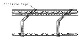
Step4: put into inner package carton ,and use adhesive tape to seal
