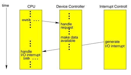
Figure 4: Timing of I/O Operations on a real machine
