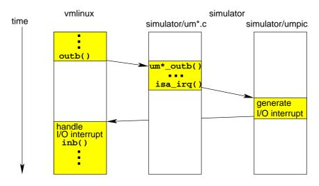
Figure 5: Timing of I/O Operations on a UMLinux machine
