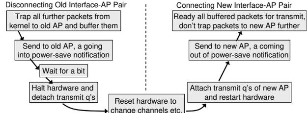
Figure 7: FatVAP’s approach to switching between interfaces
