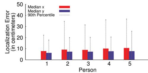
**Figure 14—Accuracy for Localizing Breathing People in Line-of-Sight.** The figure shows show the median and 90<sup>th</sup> percentile errors in x/y location. Subjects are ordered from first to last detected by SSC.
