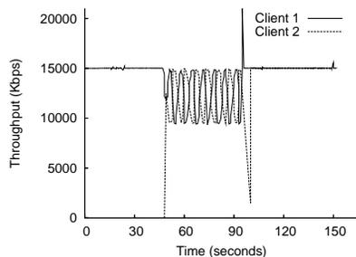
**Figure 19. Load balancing: 2 CBR UDP flows**
