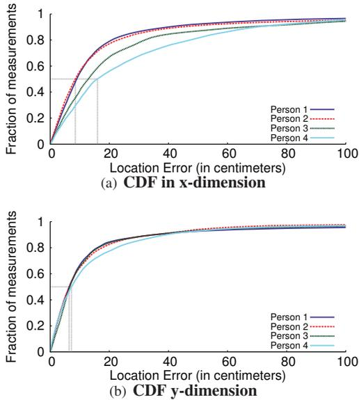
**Figure 12—Performance of WiTrack2.0's LOS Tracking.** (a) and (b) show the CDFs of the location error in x and y for each of the tracked users in LOS. Subjects are ordered from first to last detected by SSC.
