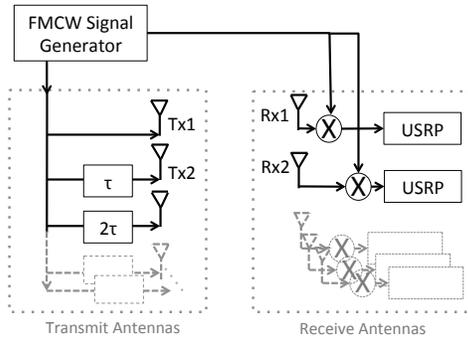
**Figure 5—Multi-shift FMCW Architecture.** The generated FMCW signal is fed to multiple transmit antennas via different delay lines. At the receive side, the TOF measurements from the different antennas are combined to obtain the 2D heatmaps.
