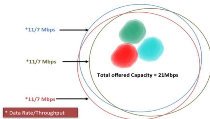
**Figure 7. 21 Channels on One 5 GHz Cell, and Resulting Capacity**
