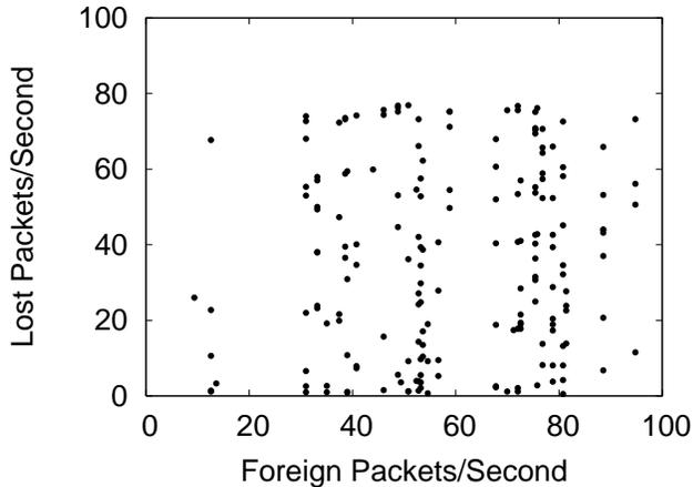
**Figure 18:** Each point indicates one host pair. The  $x$ -axis shows the number of foreign packets received per second by the receiver in that pair (same data as Table 1). The  $y$ -axis shows the number of 1500-byte packets lost per second at 1 Mbit/s. The data for the two axes are from experiments performed within a few minutes of each other. There is no obvious correlation.
