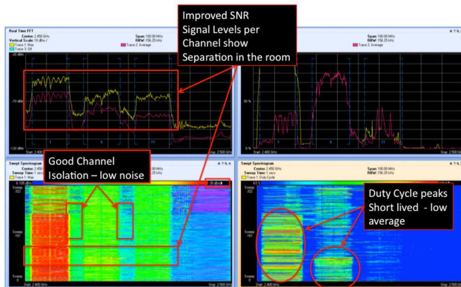
Note that for Room A the scale of the swept spectrogram in the lower left corner of the display had the red level set to -39 dBm and in Room B it was adjusted to -50 dBm. Signals were quite a bit hotter in Room A. Room A had fewer channels and the APs were further from the client; this in turn caused the clients to increase their power. The combination of the increased power and fewer channels in roughly the same space caused more noise and faster deterioration of the overall available spectrum.
