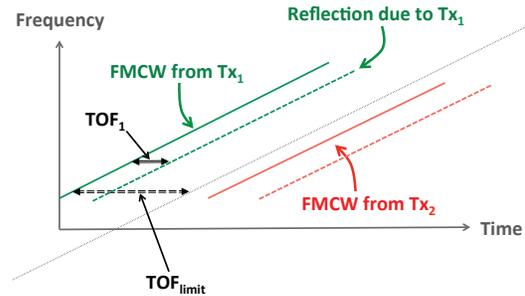
**Figure 4—Multi-shift FMCW.** WiTrack2.0 transmits FMCW signals from different transmit antennas after inserting virtual delays between them. Each delay must be larger than the highest time-of-flight ( $TOF_{limit}$ ) due to objects in the environment.
