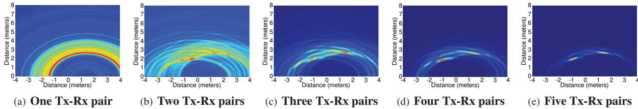
**Figure 3—Increasing the Number of Tx-Rx pairs enables Localizing Multiple Users.** The figure shows the heatmaps obtained from combining TOF profiles of multiple Tx-Rx antenna pairs in the presence of two users. The x/y axes of each heatmap correspond to the real world x/y dimensions.
