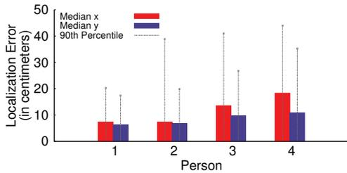
**Figure 15—Accuracy for Localizing Breathing People in Through-Wall Experiments.** The figure shows show the median and 90<sup>th</sup> percentile errors in  $x/y$  location. Subjects are ordered from first to last detected by SSC.
