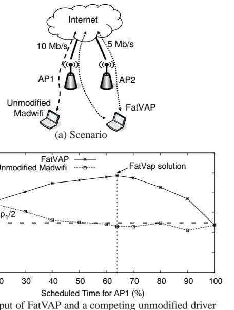
**Figure 12:** FatVAP shares the bandwidth of AP1 fairly with the unmodified driver. Regardless of how much time FatVAP connects to AP1, the unmodified driver gets half of AP1's capacity, and sometimes more. The results are for the downlink. The uplink shows a similar behavior.
