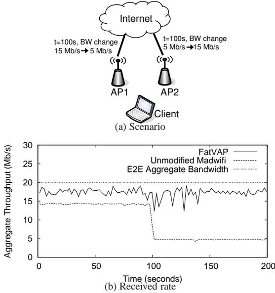
Figure 10: At time  $t = 100$ s, the available bandwidth at the first access link changes from 15Mb/s to 5Mb/s, whereas the available bandwidth at the second access link changes from 5Mb/s to 15Mb/s. FatVAP quickly rebalances the load and continues to deliver the sum of the APs’ available end-to-end bandwidth. In the scenario, an unmodified driver limits the client to AP1’s available bandwidth.
