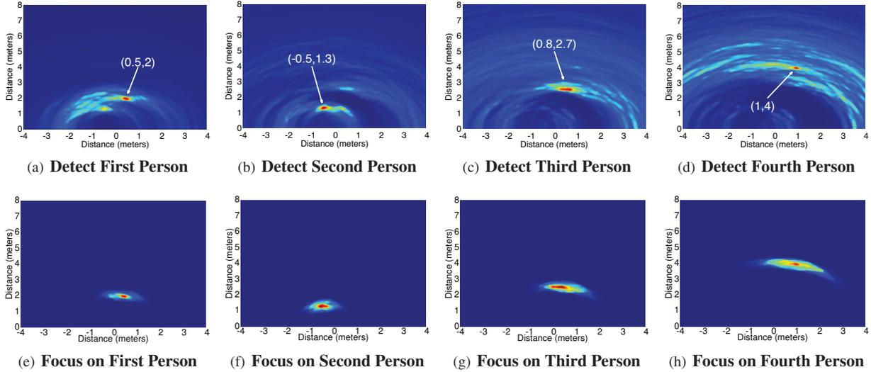
**Figure 6—Successive Silhouette Cancellation.** (a) shows the 2D heatmap obtained by combining all the TOFs in the presence of four users. (b)-(d) show the heatmaps obtained after canceling out the first, second, and third user respectively. (e)-(h) show the result of the SSC focusing step on each of the users, and how it enables us to accurately localize each person while eliminating interference from all other users.
