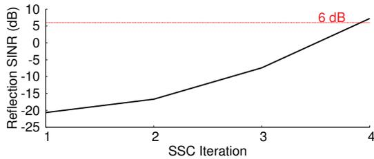
**Figure 8—SINR of the Farthest User Throughout SSC Iterations.** The figure shows how the SINR of the farthest user increases with each iteration of the SSC algorithm. After the first, second and third person are removed from the heatmap images in Figs.6(a)-(c), the SINR of the fourth person increases to 7dB, allowing us to detect his presence.
