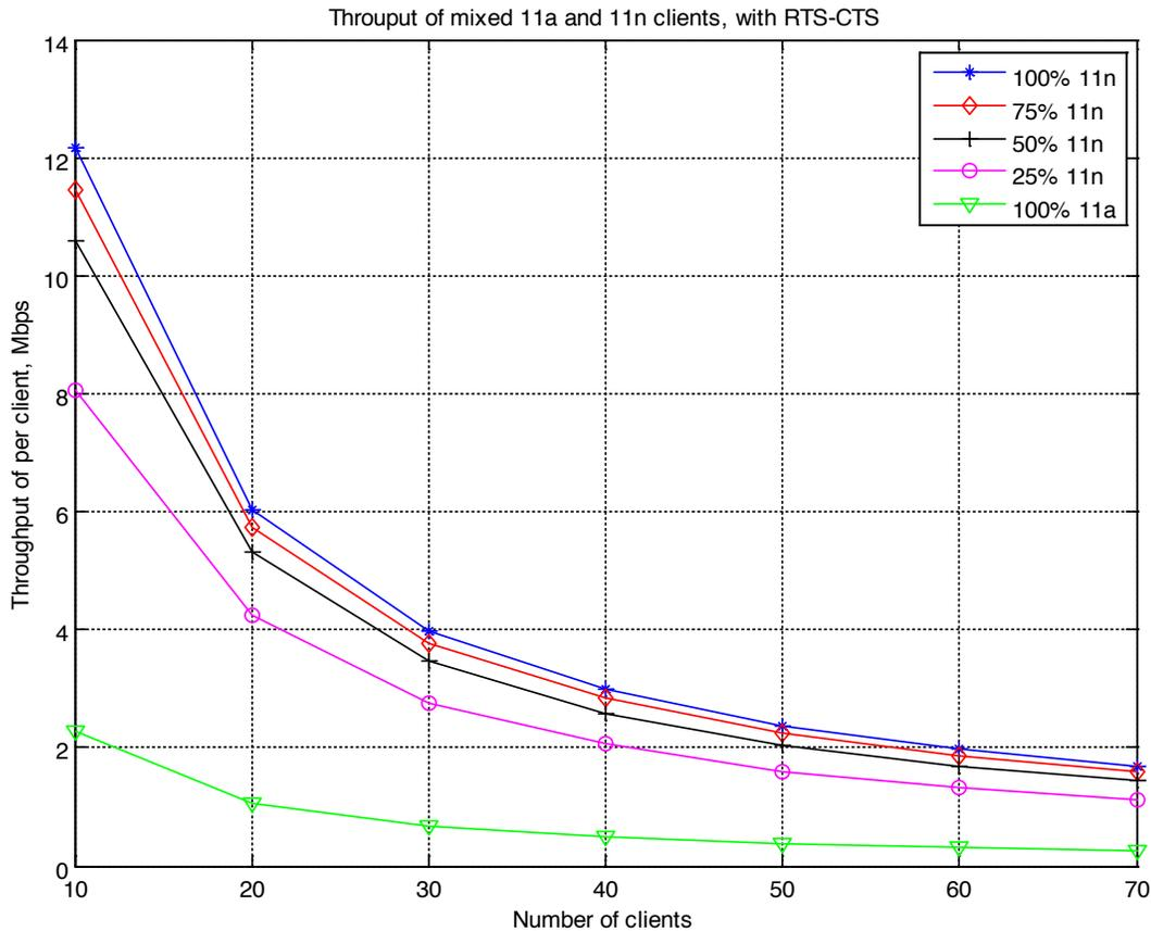
The graph above shows throughput rates under varying mixes of HT20 modulation coding scheme-15 (MCS15) 2SS data rates and legacy 802.11a/g (for the purpose of this discussion 802.11a and 802.11g are the same protocol – different bands and are considered equal) data rates within a single isolated cell.
