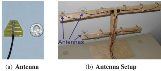
**Figure 2—WiTrack2.0’s Antennas and Setup.** (a) shows one of WiTrack2.0’s directional antenna ( $3\text{cm} \times 3.4\text{cm}$ ) placed next to a quarter; (b) shows the antenna setup in our experiments, where antennas are mounted on a  $2\text{m} \times 1\text{m}$  platform and arranged in a single vertical plane.
