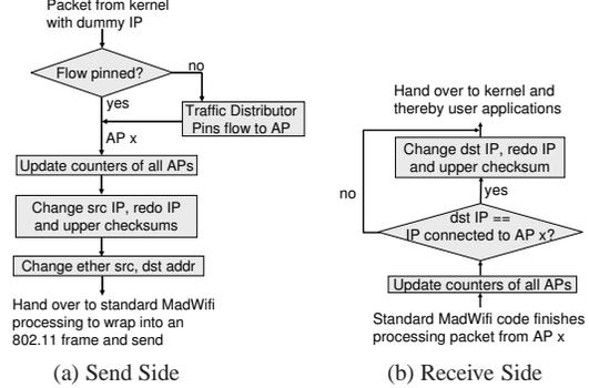
**Figure 6:** Getting packets to flow over multiple interfaces.
