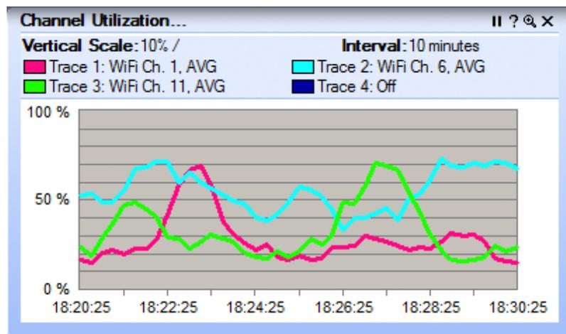
The duty cycle measures the actual RF utilization; it is the percentage of time Tx is active for a given frequency. Channel utilization is different, and normally a higher value than RF duty cycle as it adds protocol timers into the metric to show overall Wi-fi channel availability. By adding the contention window minimum (CW\_min), network allocation vector (NAV) and CCA high
