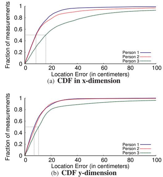
**Figure 13—Performance of WiTrack2.0's Through-Wall Tracking.** (a) and (b) show the CDFs of the location error in x and y for each of the tracked users. Subjects are ordered from first to last detected by SSC.
