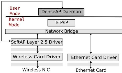
Figure 5. The network stack on each DenseAP node
