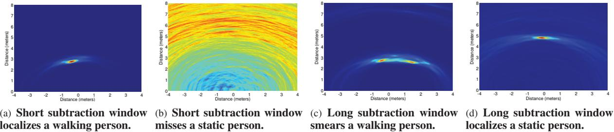
**Figure 10—Need For Multiple Subtraction Windows.** The 2D heatmaps show that a short subtraction window accurately localizes a pacing person in (a) but not a static person in (b). A long subtraction window smears the walking person’s location in (c) but localizes a breathing person in (d).
