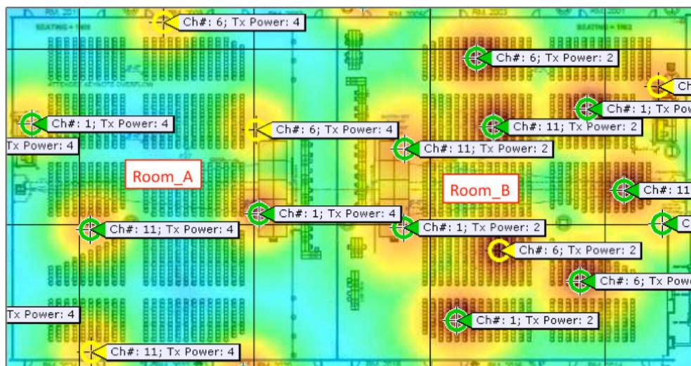
Room A has a total of six APs deployed. Two APs have directional antennas used from the sides, two APs with internal antennas are positioned at the front, one internal antenna AP is positioned at the rear of the room, and one internal AP is floor mounted to fill in for a shadow behind a pillar in the room. Power levels are set to 11 dBm and result in good coverage levels for the room. Minimum data rates are set to 9 Mbps. BandSelect and Cisco ClientLink are enabled.
