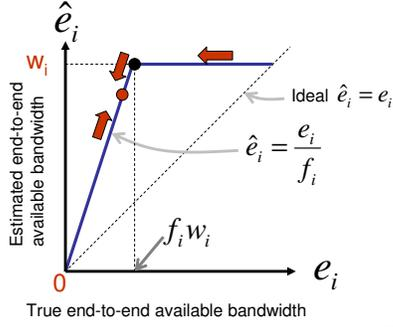
**Figure 4:** The estimate of end-to-end available bandwidth is different from the true value because the AP buffers data when the client is not listening and buffered data drains at the wireless available bandwidth. FatVAP corrects for this by spending slightly longer than necessary at each AP, i.e., operating at the red dot rather than the black dot.
