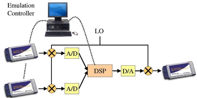
**Figure 3: Architecture of the hardware channel emulator.**
