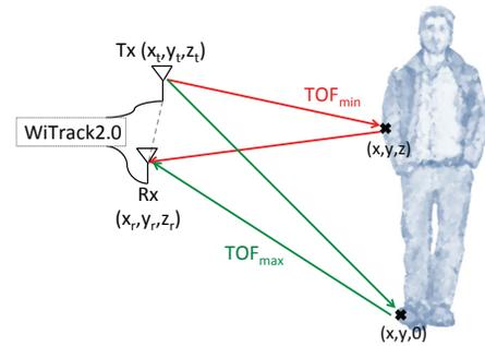
**Figure 7—Finding  $TOF_{min}$  and  $TOF_{max}$ .**  $TOF_{min}$  is determined by the round-trip distance from the Tx-Rx pair to the closest point on the person's body. Since the antennas are elevated,  $TOF_{max}$  is typically due to the round-trip distance to the person's feet.
