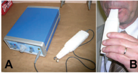
Fig. 1: First-generation neuroelectrostimulation device consisted of a hand-held probe, tipped with stainless steel electrodes, and a console that housed a battery and the electronic signal-generating power source, the size and shape of which were similar to a video or CD player
