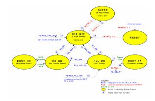
Figure 1. Basic State Machine for the RFA1 transceiver
