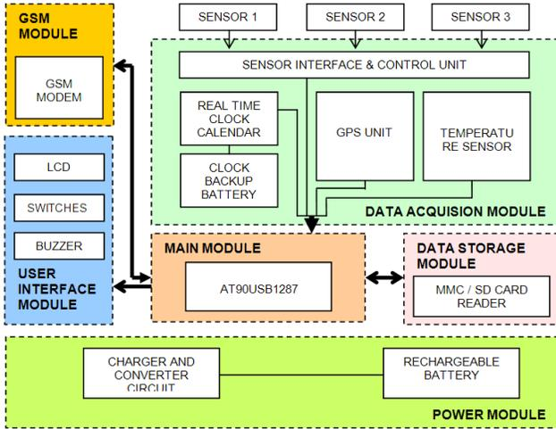
Figure 2. Mobile Unit hardware diagram.
