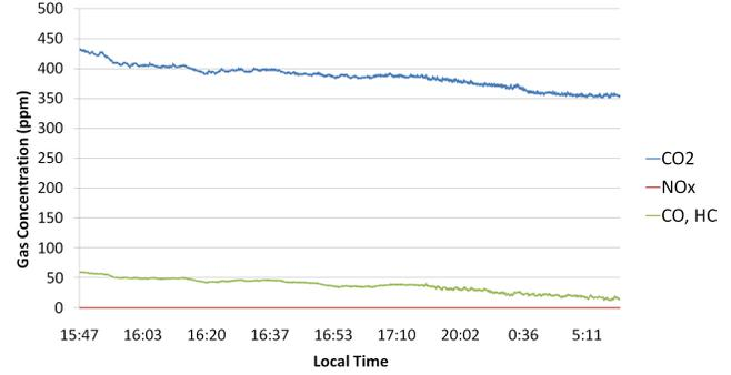
Figure 4.  $CO_2$ ,  $NO_x$  and  $CO/HC$  gas concentration variation for a fixed location
