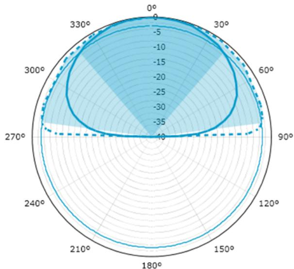
Figure 6. Total antenna gain patterns in polar and Cartesian coordinates.
