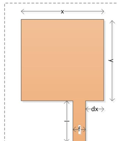
Figure 5. Dimension specifications for an edge feed patch antenna.
