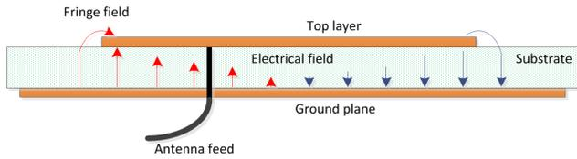
Figure 2. Patch antenna diagram.
