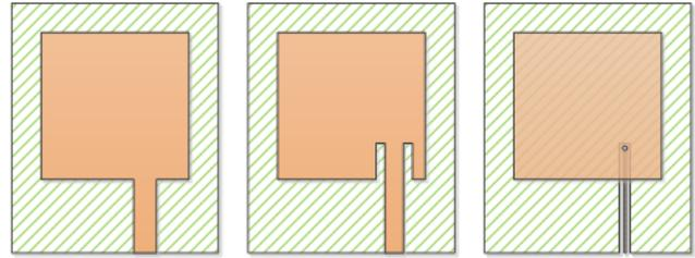
Figure 4. Different types of feeds for rectangular microstrip antennas. From left to right: edge feed, inset feed and probe feed.
