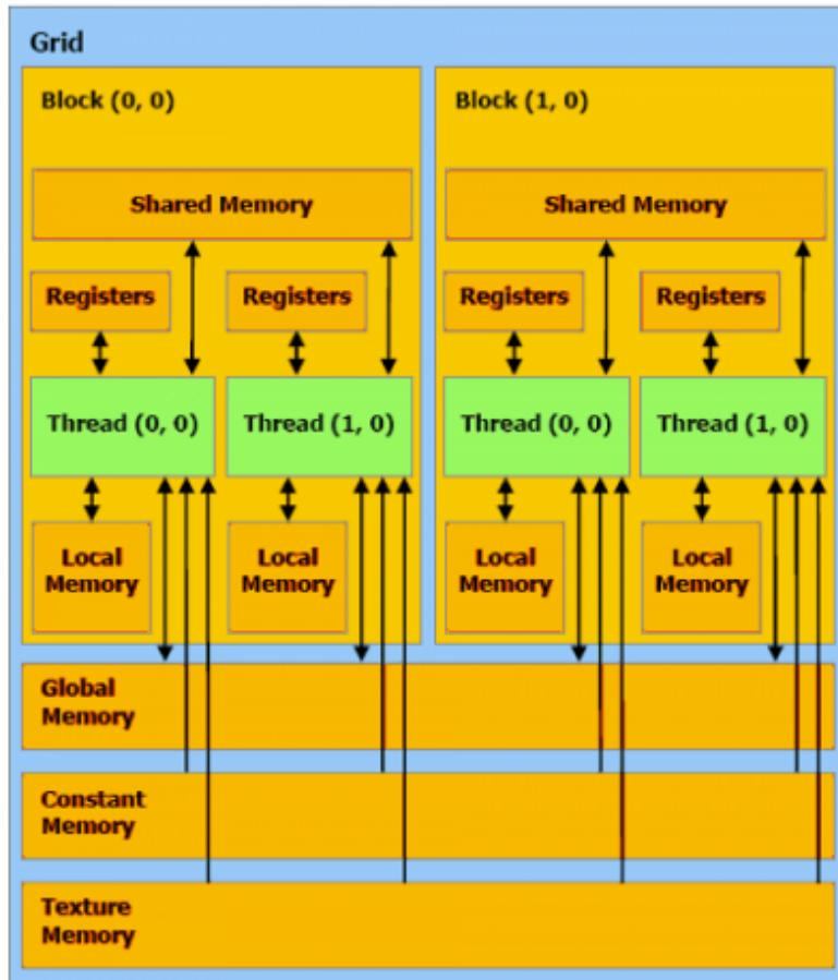
Caracteristici relevante ierarhie memorie dpdv API OpenCL, platforma NVIDIA, device Tesla M2070:
