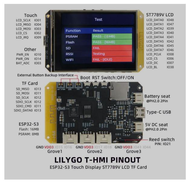
The buzzer, buttons, and joystick will be connected to the I/O pins. (IO15, IO16, IO17, IO18, IO43, IO44).
