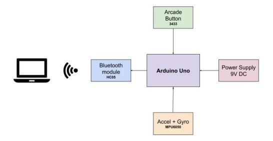
The MPU6050 communicates with the Arduino Uno via the I2C protocol. The Arduino processes the data and transmits it via UART to an HC05 Bluetooth module. On the PC side, a program receives the Bluetooth data and emulates keyboard input, making the glove behave like a motion-enabled controller.
