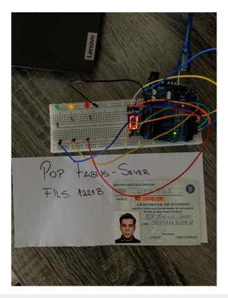
I have successfully created a functional traffic light controller. The signals from the microcontroller were transmitted correctly to the LEDs, and the 7-segment display showed the corresponding number of seconds for the time interval. I have obtained a product that functions according to the specifications and can be used to control a traffic light.
