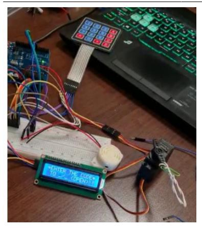
Components: \* **All of them were from https://www.optimusdigital.ro/**\* \* Arduino UNO R3 Compatible Development Board (ATmega328p + ATmega16u2) + 50 cm Cable \* Servo Motor S3003 \* 4×4 Matrix Keypad \* 1602 LCD with I2C Interface and Blue Backlight
