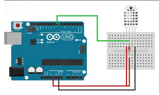
After connecting both the I2C LCD and DHT22 temperature and humidity sensor, the setup looks like this:
