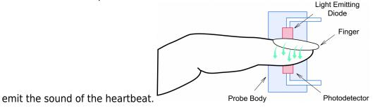
The heart rate sensor is an Arduino-compatible device that can be easily connected and used. It consists of an integrated optical amplification circuit and a noise elimination circuit to ensure accurate pulse measurement.
