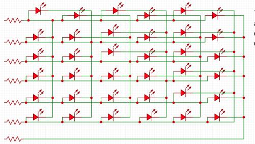
This specific configuration allows the control of the entire matrix using only 7 output pins.
